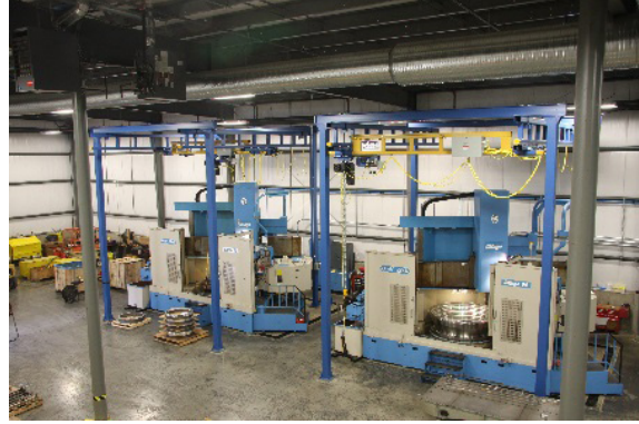
New Facility Layout: Opening up space in the new facility allowed the team to place machines closer together to reduce lag time without creating potential bottlenecks
