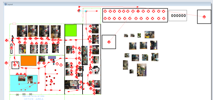
New Facility Layout: The red paths represent the forklift routes that have been placed to ensure aisle way requirements have been met for forklift movement and maintenance
